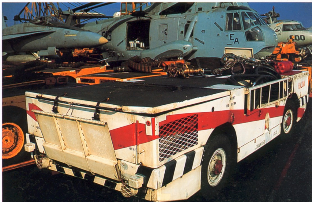
Fig.3 The small foldable platform and handhold bar at the rear of the tractor. Note the engine deck does not fit tightly and is held in place with rubber tie-downs.
