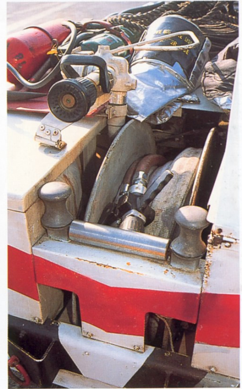
Fig.7 A large reel is located in the middle and is flanked by rollers to guide the hose while unwinding.
