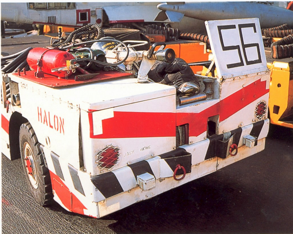
Fig.6 Layout and markings of the front including the red painted V and bumper stripes as well as the black 56 on the driver's protective shield. Also note the reflectors (for nighttime operations) and the tie-down rings.
