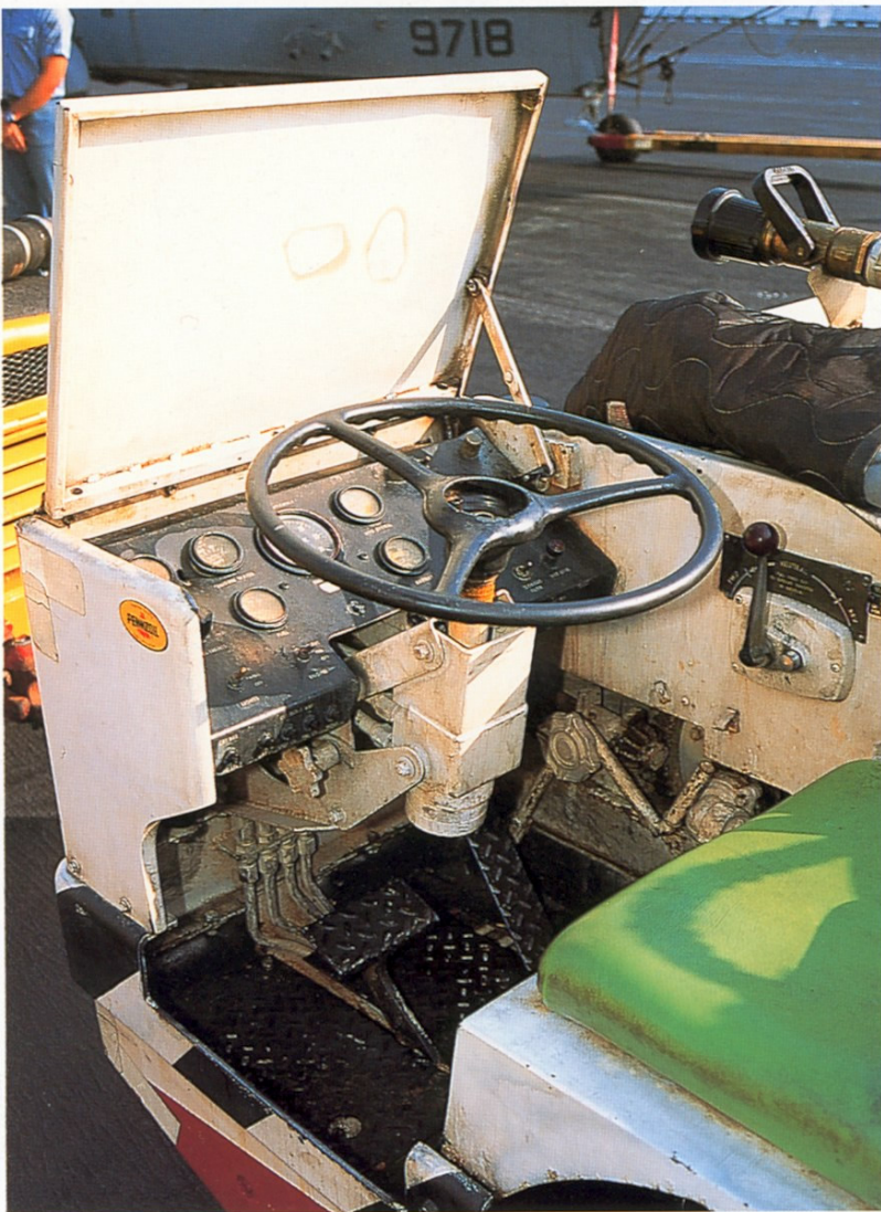
Fig.4 The driver's position with steering wheel and operating pedals. Note the way the steering wheel is attached to the control column and the operating lever on the right.
